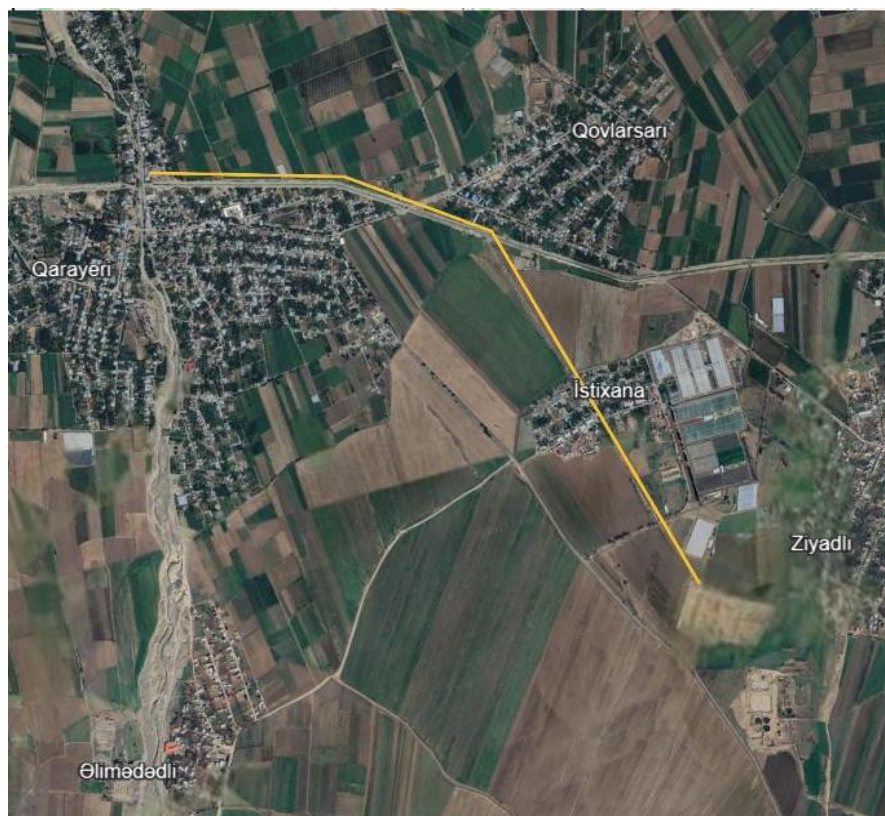
Figure 3. Proposed effluent discharge pipeline route from Ganja WWTP to irrigation canal and river 3
